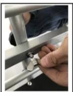
Step 4: Assemble the tow bar to the trailer frame by using the two knobs . Locked it by using gasket and butterfly knobs..Now your trailer is ready for use.
