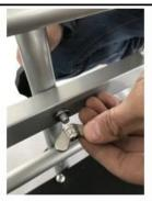
Step 8: Assemble the tow bar to the trailer frame by using the two knobs (F). Locked it by using gasket and butterfly knobs.
