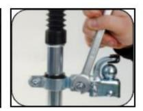
Step 9: Secure the saddle-support mounting, with the help of the plastic shims (17), to the saddle pillar of your bicycle.
